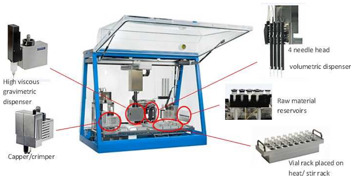
Figure 2. Image of “Swing Emulsifier” platform and robotic tools used for the microemulsion formulations
