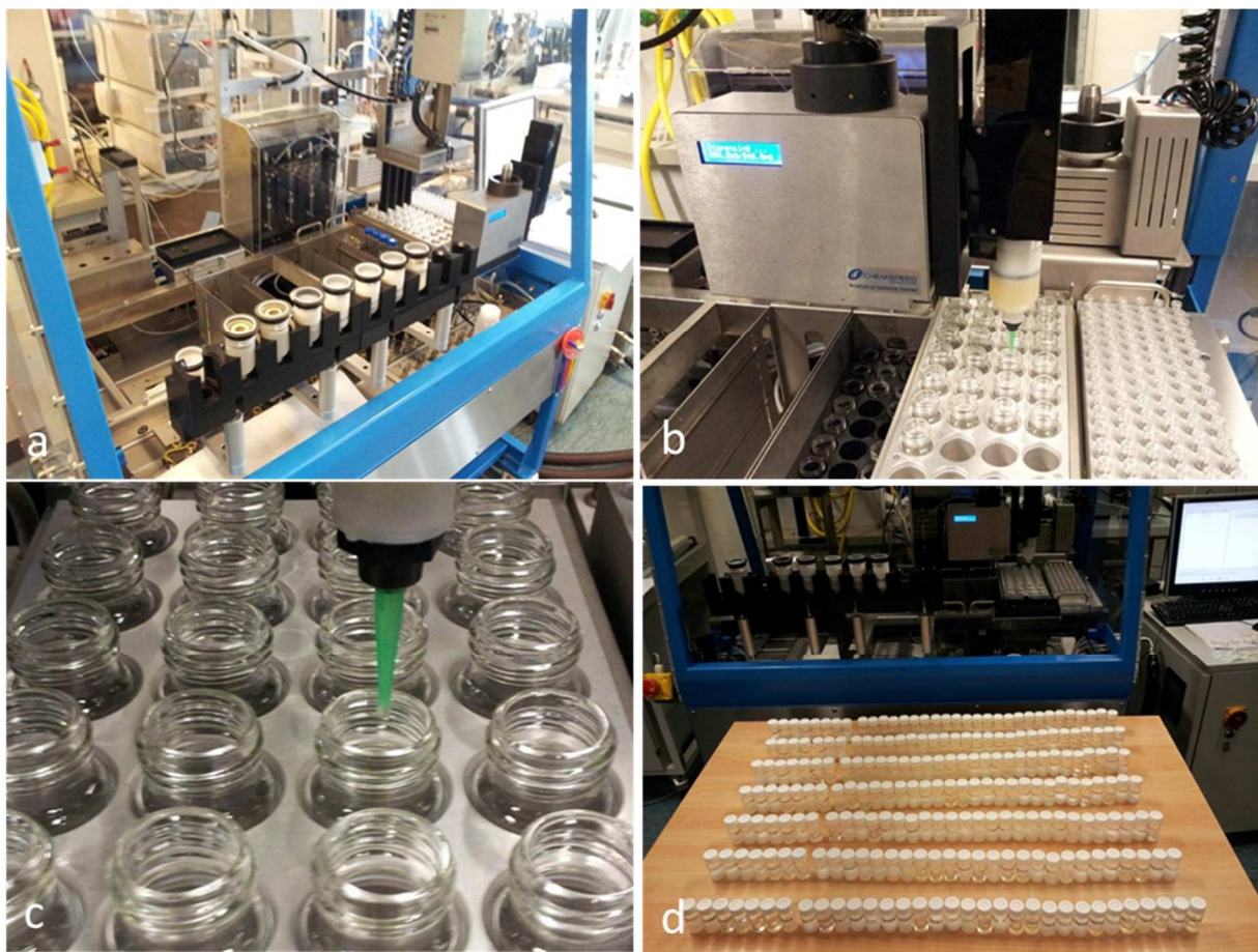
Figure 3. Image of a) the used “Swing Emulsifier” platform, b) the dispensing unit, c) close up of the dispensing unit and d) all samples which have been prepared
