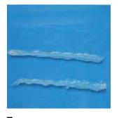
Silicon sealant was easy to peel off – adhesion failure.
