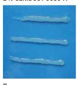
Unable to remove sealant – cohesion failure.
