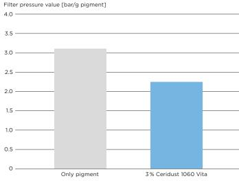
Formulation: Polylactic acid + 30 % Blue 15:3 + indicated percentage of test product Filter value: DIN-EN 13900-5; Filter: 14 µm; Premix: Cold mix
