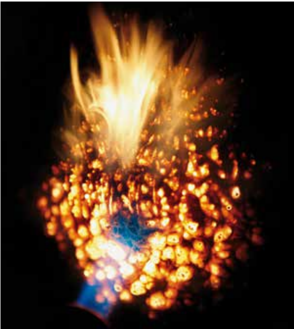
The intumescent effect can be demonstrated with a Bunsen burner.
