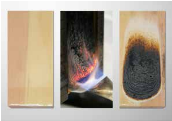
— Performance of a fire protection coating on wood with Exolit 855.
